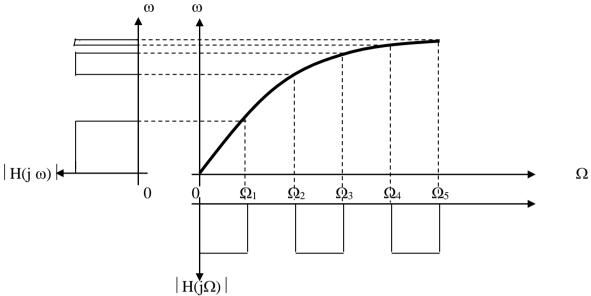
The relation between analog frequency and digital frequency is non linear. When the s-plane is mapped into the z-plane using bilinear transformation, the non-linear relationship introduces the distortion in frequency axis with disproportionate bandwidth is called frequency warping.
