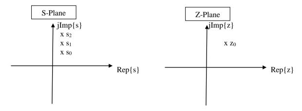
Impulse invariant transformation is a many-to-one type of conversion or mapping method, because it maps many poles in s-domain into single pole in z-domain. Effect of getting single digital frequency for various analog frequencies is known as frequency aliasing.
